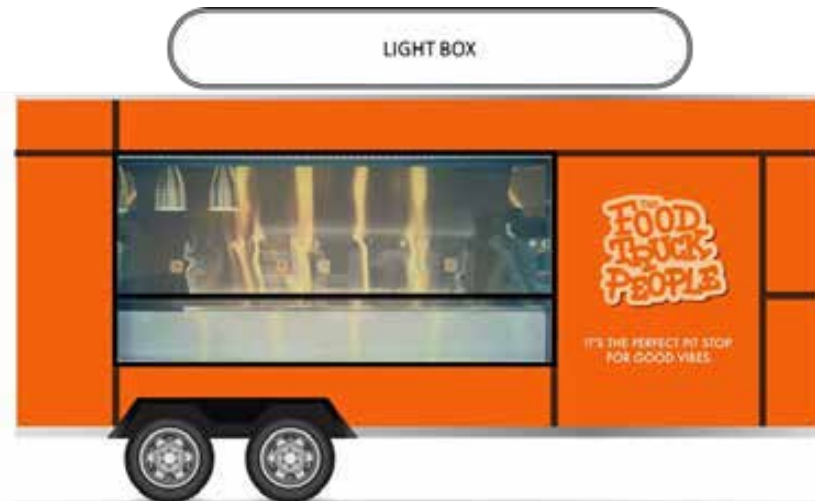
Trailer 3- Cabin : 4.8m (L) x 2.1m (W) x 2.8m(H) with lightbox & excluding trailer rod
